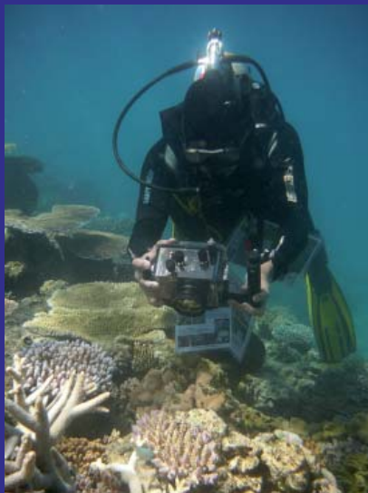
Sampled coral colonies are photographed, and the time-stamps of the digital images are used for identifying the geocoordinates of the sample from the tracklog taken by a GPS buoy above the diver
